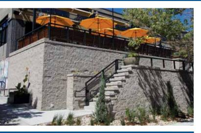
Multiple Face Designs • Near-Vertical or Battered Setback Installation • Tall Walls • Critical Structures
