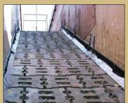
SHOREBLOCK® SD has been successfully tested by Colorado State University, in accordance with the hydraulic performance testing protocol established by the U.S. Federal Highway Administration.
