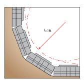
Each block is interconnected by flexible cables, providing articulation between adjacent blocks.
