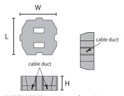
SHOREBLOCK® BD units are manufactured in accordance with ASTM C90, C140 and D6684-04 and the following criteria: concrete unit weight 130-150 lbs./CF, minimum compression strength 4,000 PSI, Maximum Absorption 7% and dimensional tolerance  $\pm$  1/8".
